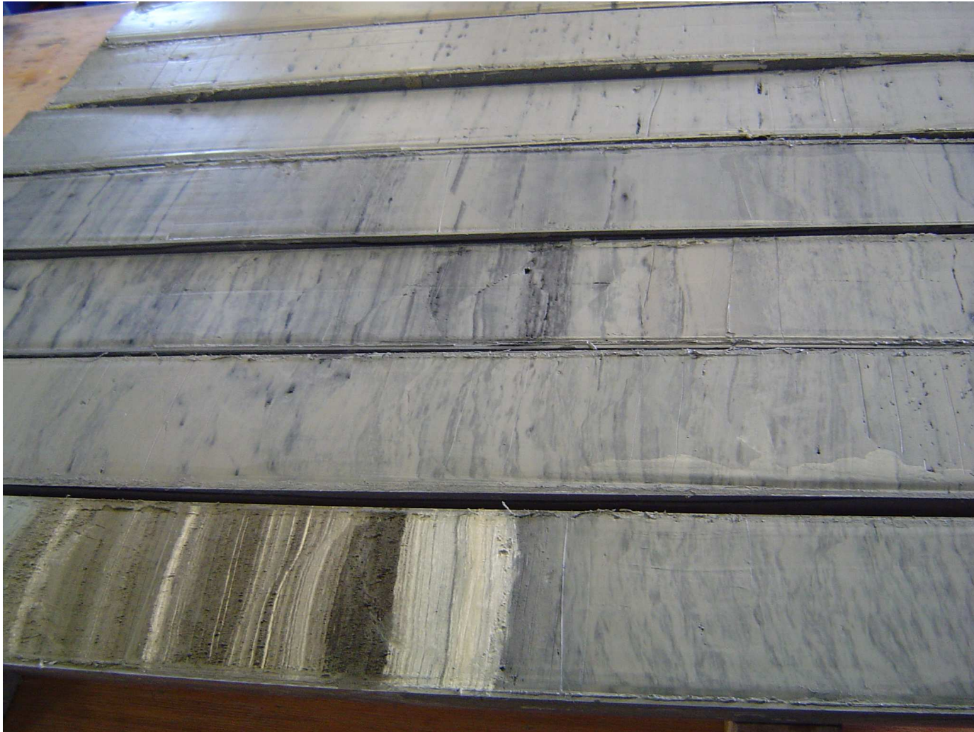
Gravity core from the Black Sea with limic (black greigite banding) and marine sapropel (Eemian) sequences. (© 2009, Max Planck Institute for Marine Microbiology)
